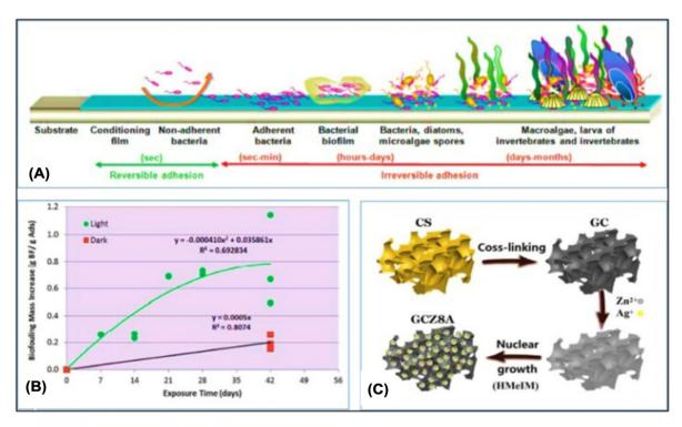
Fig. 10 (A) Marine fouling development methods. 187 (B) Elevation in the dry mass of the biofouling material with time in both light and dark streams. Biofouling mass is a representation of the biofouling material accumulated during 42 days (g)<sup>188</sup> per adsorbent mass (g). (C) Illustrative GCZ8A composites synthesis schematic proposed. 56
