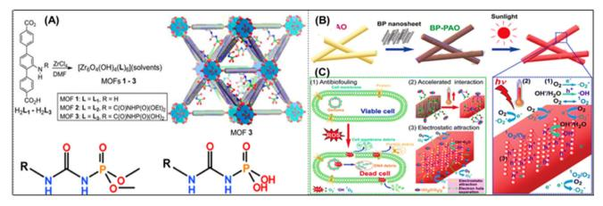
Fig. 5 (A) Diagram illustrating the combination of 1–3. (Bottom) Right and left 1 and 2 have orthogonal functionalities. (B) Diagrammatic representation of the BP-PAO fibre preparation process. (C) Mechanism of the BP-PAO fiber uranium absorption and antifouling. (B) Diagrammatic representation of the BP-PAO fibre preparation process.
