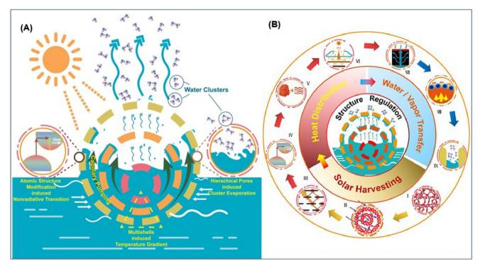
Fig. 9 (A) Illustration of the very efficient solar-to-vapor production method using amorphous  $Ta_2O_5/C$  HoMS of amorphous  $Ta_2O_5/C$  HoMS for highly efficient solar-to-vapor production. 176 (B) Regulation of the solar vapor generating structure affects each of the subsequent processes in the process, such as heat distribution, water/vapor transfer, and solar harvesting. 194
