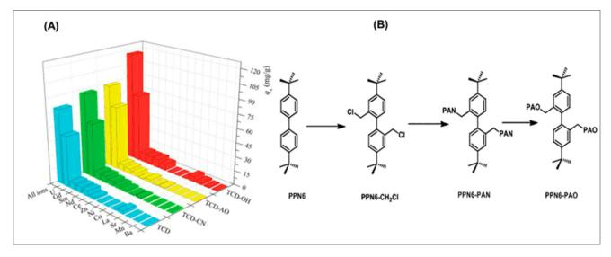
Fig. 6 (A) The effectiveness of TCD COF and its derivatives in the aqueous solution for the selective recovery of uranium over 11 other competing ions. The experiment was run for three hours at 25 °C and pH 4.5. At first, each metal was introduced at a concentration of 0.5 mmol  $L^{-1.123}$  (B) Method for generating amidoxime-functionalized POP synthetically (PPN-6-PAO). <sup>138</sup>
