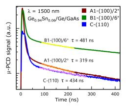
Fig. 8 μ-PCD signal versus time acquired at 300 K with 1500 nm excitation wavelength from samples A1 [(100)/2° Ge<sub>0.94</sub>Sn<sub>0.06</sub>], B1 [(100)/6°  $\text{Ge}_{0.94}\text{Sn}_{0.06}]$  and C [(110)  $\text{Ge}_{0.94}\text{Sn}_{0.06}].$  The corresponding minority carrier lifetimes of ~319 ns, ~481 ns and ~434 ns were obtained by fitting to exponential decay after the initial surface recombination induced decay.
