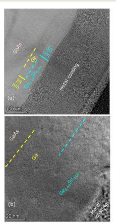
Fig. 5 Cross-sectional TEM micrographs of sample A2: (a) Ge<sub>0.94</sub>Sn<sub>0.06</sub>/ Ge/(100)/2° GaAs heterostructure representing good quality growth of 50 nm  $Ge_{0.94}Sn_{0.06}$  grown over 38 nm thick Ge layer grown on GaAs, where broken lines demarcate similar structure factored Ge and Ge<sub>0.94</sub>Sn<sub>0.06</sub> epilayers, and (b) HR-TEM micrograph affirms the fine quality of the GeSn/Ge heterostructure system.
