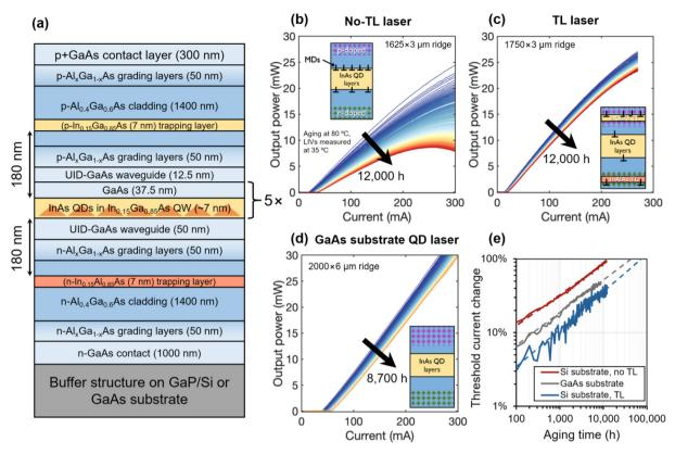
Fig. 1 (a) Schematic of laser structure with trapping layers. (b–d) Light output vs. current (L-I) measurements over the course of aging for the three lasers: (b) on silicon without trapping layers (12 000 h), (c) on silicon with trapping layers (12 000 h), and (d) on GaAs substrate (8700 h). (e) Laser degradation rates measured by increase in threshold current. Extrapolated lifetimes (100% increase in threshold current) are indicated with the dashed lines
