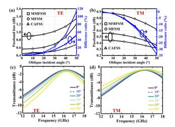
Fig. 7 (a)–(b) Passband loss and difference ratio *versus* incidence angle of CAFSS, MFSM, and MMFSM under (a) TE polarization and (b) TM polarization. (c)–(d) Simulated transmittance of the MMFSM for different incidence angles under (c) TE polarization and (d) TM polarization.
