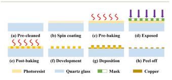
**Fig. 8** Fabrication process of the FSM sample: (a) pre-cleaning; (b) spin coating; (c) pre-baking; (d) exposure; (e) post-baking; (f) development; (g) deposition; (h) peeling off.
