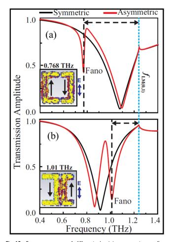
Fig. 10 Fano resonances of different aluminium resonator configurations. (a) Square configuration of end-coupled resonator arms and (b) side-coupled configuration with the resonating arms flipped. Reproduced from ref. 59 with permission from [John Wiley and Sons], copyright [2020].
