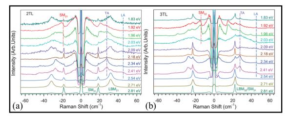
Fig. 8 (a) Ultra-low frequency Raman spectra of 2TL and (b) 3TL WS<sub>2</sub> samples with different laser excitation energy ( $E_L$ ). Reproduced from ref. 47 with permission from [IOP Publishing], copyright [2014].
