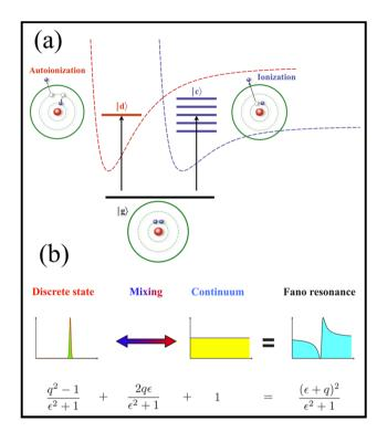
Fig. 1 (a) Schematic representation of Fano resonance and (b) a schematic depiction of the Fano formula (egn (1)) in terms of its components as the interference of discrete states with electronic continuum. Reproduced from ref. 29 with permission from [American Physical Society], copyright [2010].
