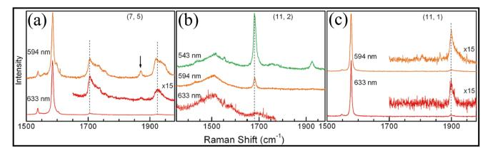
Fig. 6 Excitation wavelength-dependent Raman spectra of three individual tubes: (a) semiconducting tube (7, 5), (b) metallic tube (11, 2), and (c) semiconducting tube (11,1). Spectra were acquired using laser wavelengths of 633, 594, and 543 nm. Arrow in panel a indicates the weak G + RBM combination feature. All spectra are normalized to the G band peak of each tube. Reproduced from ref. 51 with permission from [American Chemical Society], copyright [2009].
