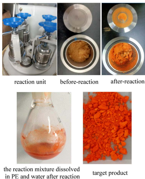
Fig. 1 Ball milling setup and process.
