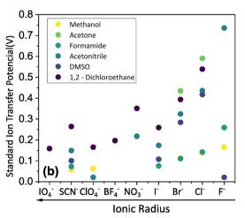
Fig. 4 (a) Effect of  $\gamma$  variation on output curve shape. Here were used the following parameters w = 1.5 mm, h = 100 nm, l = 250 um,  $\sigma = 1.5$  S cm $^{-1}$ .  $\sigma_{res}$  = 1  $\times$  10<sup>-4</sup> S cm<sup>-1</sup>,  $\mathcal{E}_{pol}^{\ominus'}$  = 0 V, T = 298.15 K,  $\Delta V_{gs}$  = -0.5 V. (b) Standard Ion Transfer Potential for anions from water to organic solvent from ref. 66-68 with adaptations
