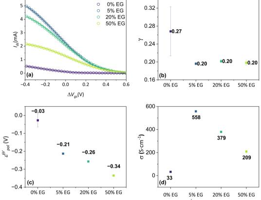
Fig. 6 (a) Transfer curves (hollow circles) from Rivnay (2016), and fitting curves (solid lines), (b)  $\gamma$ , (c)  $\mathcal{E}_{pol}^{\ominus}$  and (d)  $\sigma$  parameters. Reprinted (adapted) with permission from Rivnay *et al.* (2016).<sup>47</sup> For all adjustments  $R^2 = 0.99$  and p-values < 0.05.
