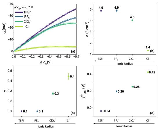
Fig. 5 (a) Output curves (hollow circles) from Flagg (2018), and fitting curves (solid lines) (b)  $\sigma$ , (c)  $\gamma$  and (d)  $\mathcal{E}_{pol}^{\ominus'}$  parameters. Reprinted (adapted) with permission from Flagg et al. (2018).<sup>26</sup> Copyright © 2018, American Chemical Society. All data fittings with R<sup>2</sup> = 0.99 and p-values < 0.05.
