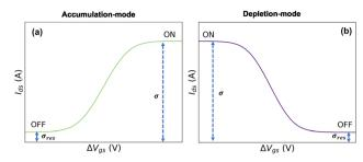
Fig. 2 Representation of residual conductivity from transfer curves for (a) accumulation-mode OECT and (b) depletion-mode OECT.
