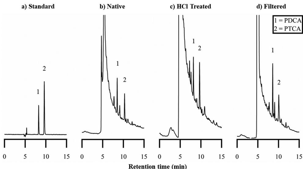
Fig. 8 High-performance liquid chromatography (HPLC) chromatograms of (a) standard eumelanin markers, and AHPO mixtures from (b) original native BSF eumelanin, (c) HCl-AHPO mixtures from BSF eumelanin and (d) AHPO mixtures from 0.2  $\mu\text{m}$  filtered BSF eumelanin.
