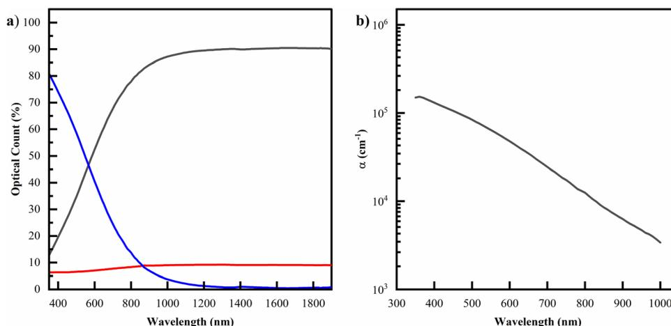
**Fig. 3** (a) The optical data for samples of a filtered solution drop cast on UV-ozone treated glass. (b) The corresponding modelled absorption coefficient. Datasets for the other permutations of (un)filtered and (un)treated films can be seen in the ESI.<sup>†</sup>
