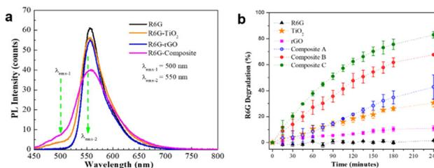
Fig. 22 (a) PL spectra and (b) photocatalytic performance of the TiO<sub>2</sub>/rGO nanocomposite. Reprinted with permission from ref. 43 Copyright 2021, the American Chemical Society.
