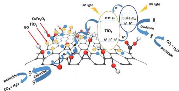
Fig. 24 Proposed mechanism describing the process of charge separation in  $\text{TiO}_2/\text{GO}/\text{CuFe}_2\text{O}_4$  through a direct Z-type scheme when exposed to UV light. Reprinted with permission from ref. 132 Copyright 2020, The Royal Society of Chemistry.
