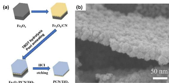
Fig. 9 (a) Illustration of  $Fe_3O_4$ -template assisted fabrication of PCN/TiO<sub>2</sub>. (b) SEM image of PCN/TiO<sub>2</sub>. Reprinted with permission from ref. 66 Copyright 2023, Elsevier.
