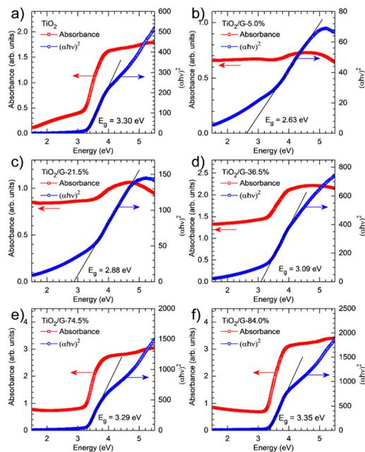
Fig. 23 UV-vis diffuse reflectance spectra and related Tauc plots of  $\text{TiO}_2$  (a) and  $\text{TiO}_2/\text{graphene}$  with varying  $\text{TiO}_2$  loadings (5% (b), 21.5 (c), 36.5% (d), 74.5% (e), and 84% (f)). Reprinted with permission from ref. 131 Copyright 2021, Elsevier.
