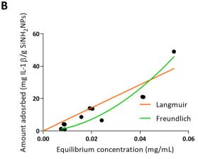
Fig. 4 Adsorption isotherms of IL-1β over SiOHNPs (A) and SiNH<sub>2</sub>NPs (B) with representation of Langmuir and Freundlich curves in orange and green, respectively
