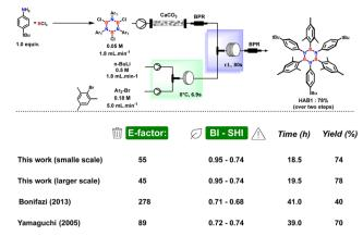
**Fig. 6** Comparison of *E*-factor, benign–safety/hazard index, reaction time and yields for this work in flow and other procedures in batch conditions.
