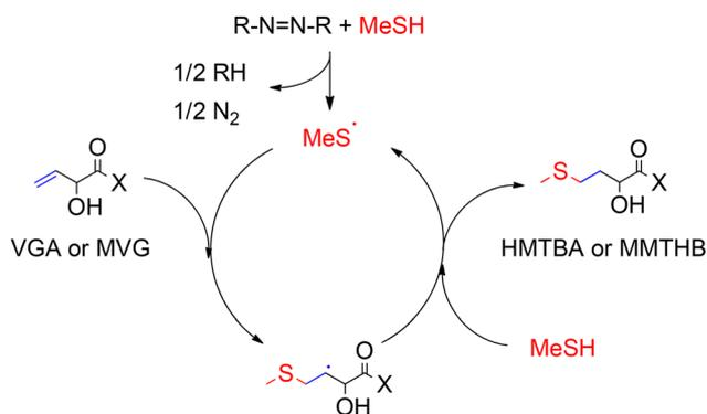
**Scheme 10** Reaction for the conversion of VGA and MVG to methionine hydroxy analogues HMTBA and MMTHB through free radical thiol-ene addition. X represents  $-\text{OH}$  or  $-\text{OMe}$  and R represents  $[(\text{CH}_3)_2\text{C}(\text{CN})]$ .
