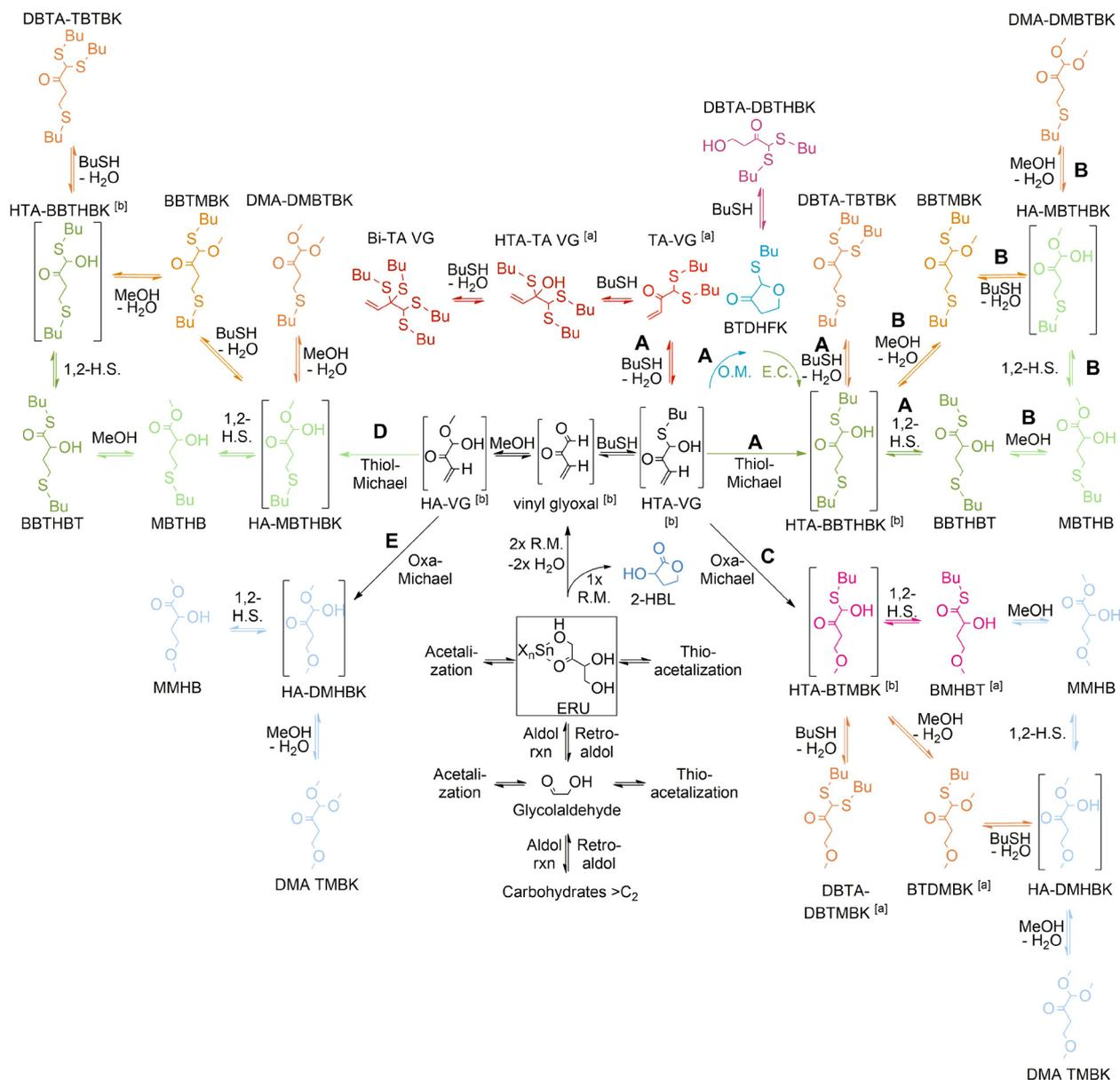
**Scheme 14** Reaction pathways for the acid-catalyzed conversion of tetroses in the presence of butanethiol and butanethiol/methanol mixtures. Reaction pathways: A (in BuSH as solvent), B and C (in BuSH rich medium), D (in BuSH poor medium) and E (in MeOH) Reproduced from ref. 134 with permission from John Wiley and Sons, copyright 2022.
