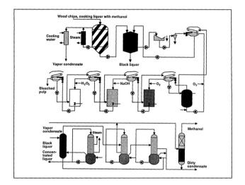
Fig. 5 The ASAM process (reproduced from ref. 72 with permission from *Tappi J.*, copyright 1991).
