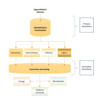
Fig. 1 Organosolv fractionation in biorefinery.
