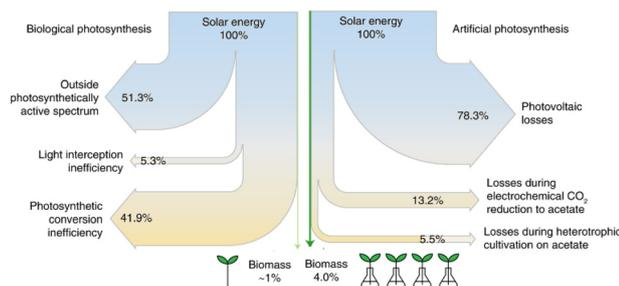
**Fig. 10** Sankey diagrams of solar energy to plant- and algae-based food production compare the efficiencies of artificial and biological photosynthesis. Adapted from Hann *et al.*<sup>182</sup> Copyright Springer Nature 2022.
