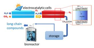
Fig. 8 In vitro artificial sugar synthesis system. CO2 was first converted to pure acetic acid through two-step electrolysis; this product was then directly fed for microorganism fermentation in a bioreactor to produce long-chain compounds, for example, glucose. In the inset: schematic illustration of CO reduction (COR) to pure acetic acid in the solid-electrolyte reactor. Original figure based on Zheng et al. 181 scheme.
