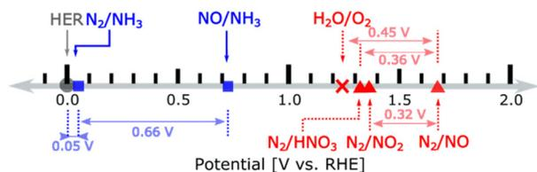
Fig. 4 Redox couples for nitrogen reduction (blue) and oxidation (red) with thermodynamic potentials. HNO<sub>3</sub> is gas. Reproduced with permission by Wan *et al.*<sup>93</sup> Copyright ACS 2022.
