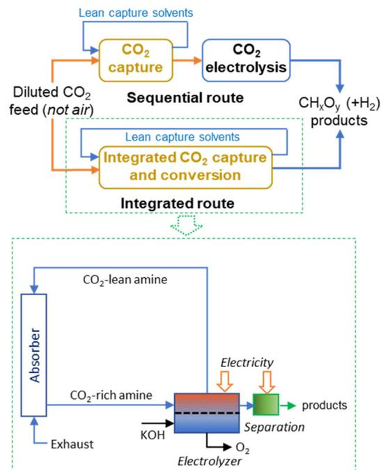
**Fig. 2** Simplified block diagrams of sequential and integrated routes for amine-based CO<sub>2</sub> capture and electrolysis with a more detailed scheme for the integrated CO<sub>2</sub> capture and direct CO<sub>2</sub> electroreduction from the capture medium. Some elements, such as the compression unit between the stripper and the electrolyser, are not shown.
