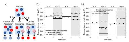
Fig. 5 (a) Schematic representation of the charge-balancing mechanisms. Calculated transmission for counter-ion adsorption (full line), ion exchange (dash-dotted line) and co-ion expulsion (dotted line) as well as measured transmission (triangular symbols) for X-ray energies of (b) 12.7 keV and (c) 14.4 keV.
