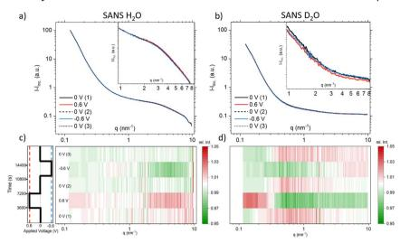
Fig. 4 Coherent SANS scattering curves and corresponding heat-plots displaying relative intensity changes for  $H_2O$  (a) and (c), and  $D_2O$  (b) and (d).
