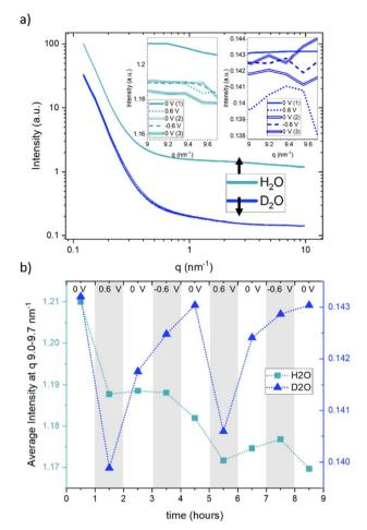
Fig. 3 SANS curves (a) and average SANS intensity in the q-range from  $9.0-9.7~{\rm nm}^{-1}$  (b) for H<sub>2</sub>O (light-blue rectangles) and D<sub>2</sub>O (dark-blue triangles). The insets in (a) show the scattering intensity in the q-range of  $9.0-9.7~{\rm nm}^{-1}$ .
