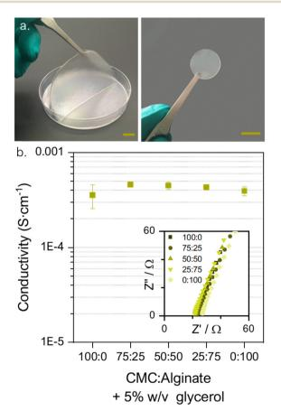
Fig. 3 Self-standing hydrogel membranes from carboxyl-methyl cellulose (CMC) and sodium alginate (AL) with 5% w/v glycerol as a plasticizer. (a) Real photographs of the 75CMC:25AL membrane. Scale bar: 0.5 cm. (b) Ionic conductivity study in relation to the biopolymers ratios and Nyquist plot (inset). N = 3
