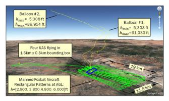
Fig. 20 Wide view in Google Earth with 2 balloon traces (yellow) and multiple rectangular aircraft patterns from a manned Foxbat (green) at different elevations. The four small drones flew concurrently within the small rectangle (blue) near the center.
