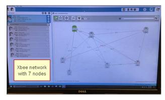
Fig. 13 Xbee mesh network view from Digi's Windows XCTU software showing 7 Xbee nodes. One node is on each of 3 multirotors and 1 fixed-wing aircraft. The others are repeater nodes to extend wireless reach, or the base station node.
