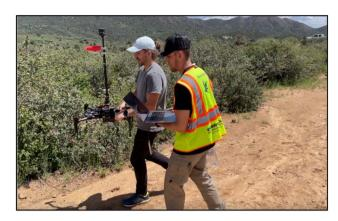
Fig. 19 Calibrating sensors on multirotor aircraft is simplest with two people: one to rotate the vehicle and the other to monitor the flight control software.
