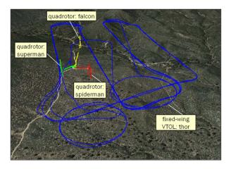
Fig. 21 The blue trace shows the fixed-wing UA flying horizontal transects with loiter circles to coordinate with three multirotors flying vertical profiles. Multirotors shown in yellow, green, and red.
