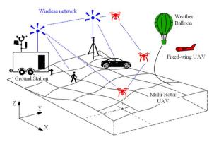
Fig. 1 Example MoVE experiment with moving aircraft (red), ground vehicles (black), pedestrians (black), and a weather balloon (green) sending telemetry data over a wireless network (blue) to a PC located in a nearby ground station.
