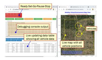
Multi-vehicle telemetry base station and monitoring displays
