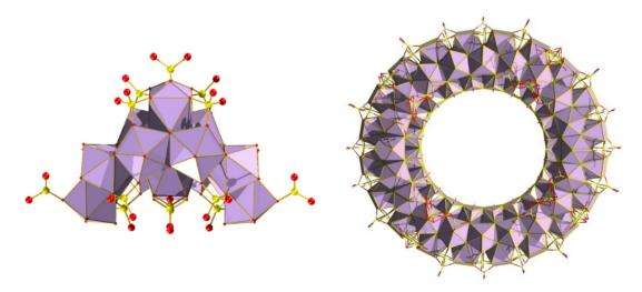
Fig. 24 Zr<sub>18</sub> cluster (left), which is isostructural to Hf<sub>18</sub>. Lowering sulfate concentration and increasing temperature led to the rearrangement to the toroidal Zr<sub>70</sub> cluster (right, top-down view). Colour code: Zr, light purple; S, yellow; O, red. Counter ions and solvate omitted for clarity.
