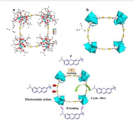
Fig. 15 (a)  $[Ti_6O_3(O^iPr)_{14}(TTFTC)]_4$ , (b) cyclic ring structure of  $[Ti_6O_3(O^iPr)_{14}(TTFTC)]_4$ , (c) suggested mechanism for the adsorption of MB. Hydrogen atoms are omitted for clarity. This figure has been adapted/reproduced from ref. 16 with permission from American Chemical Society, copyright 2022.
