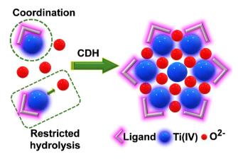
Fig. 3 Coordination-delayed-hydrolysis (CDH) method.
