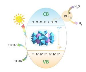
Fig. 13 Photocatalytic  $H_2$  production by the  $Ti_{21}$  cluster. This figure has been adapted/reproduced from ref. 85 with permission from Wiley-VCH GmbH, copyright 2023.
