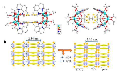
Fig. 16 (a) The structure of [Ti<sub>6</sub>O<sub>6</sub>(O<sup>i</sup>Pr)<sub>8</sub>(TTFTC)(phen)<sub>2</sub>]<sub>2</sub>, (b) TOC-MOF formed by condensation of isopropanol groups. Hydrogen atoms are omitted for clarity. This figure has been adapted/reproduced from ref. 89 with permission from American Chemical Society, copyright 2024.
