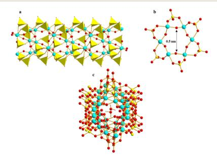
Fig. 17 (a)  $Ti-SO_4-Ti$  nanotube array of  $[Ti_6O_6(\mu_2-OH)_3(SO_4)_6]_n$ , (b)  $[Ti_6O_6(SO_4)_6]$  hexagonal hole, (c) water molecule nanoconfinement within the pores of the Ti-O nanotubes. Colour codes: Ti, cyan; S, yellow; O, red; H, white; SO<sub>4</sub>, yellow polyhedron.
