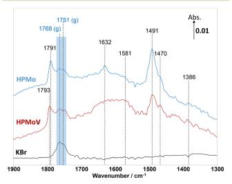
Fig. 4 Comparison of *in situ* DRIFT spectra recorded at 2 min during the adsorption of methacrylic acid (MAA) at 320  $^{\circ}$ C over  $H_3PMOO_{12}O_{40}$  (HPMo),  $H_4PMOO_{11}VO_{40}$  (HPMoV), The gas feed is composed of 3500 ppm MAA and Ar balance and the total flow rate is 100 cm³ min<sup>-1</sup>.
