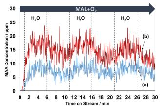
Fig. 6 Changes in gaseous MAA product as a function of time on stream at 320 °C over HPMo (a) and HPMoV (b) samples during the switches of H<sub>2</sub>O in and out of the MAL + O<sub>2</sub> gas feed. The gas feed is composed of 3500 ppm MAL, 7000 ppm O2, 7000 ppm H2O (when added), and Ar balance and the total flow rate is 100 cm<sup>3</sup> min<sup>-1</sup>.
