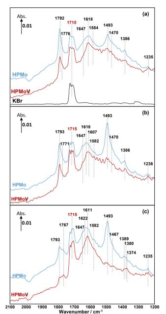
Fig. 2 Comparison of in situ DRIFT spectra recorded at 320 °C over  $H_3PMoO_{12}O_{40}$  and  $H_4PMoO_{11}VO_{40}$  at 2 min under MAL (a), MAL +  $O_2$ (b), and MAL +  $O_2$  +  $H_2O$  (c). The gas feed is composed of 3500 ppm MAL (when added), 7000 ppm O<sub>2</sub> (when added), 7000 ppm H<sub>2</sub>O (when added), and Ar balance and the total flow rate is 100 cm<sup>3</sup> min<sup>-1</sup>.
