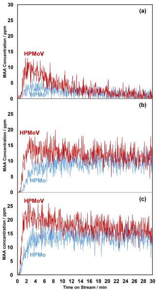
**Fig. 1** Comparison of the evolution of MAA formation at 320 °C as a function of time on stream over  $H_3PMoO_{12}O_{40}$  and  $H_4PMoO_{11}VO_{40}$  under MAL (a), MAL +  $O_2$  (b), and MAL +  $O_2$  +  $H_2O$  (c). The gas feed is composed of 3500 ppm MAL (when added), 7000 ppm  $O_2$  (when added), 7000 ppm O
