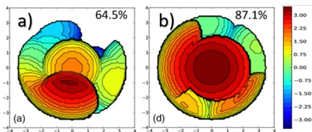
Fig. 9  $\%V_{\text{Bur}}$  and steric maps on the metal centre bonded to the halloysite: (a) without and (b) with cetrimonium bromide (*xy* plane, with the palladium placed in the centre and the *z*-axis the oxygen bonded to palladium, including the oxygen of the closest methoxy group in the *xz* plane. Curves are given in Å, with a radius of 3.5 Å).<sup>31</sup> Copyright © 2022, Wiley-VCH Verlag GmbH & Co. KGaA, Weinheim.
