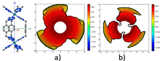
Fig. 4 Steric maps (plane  $xy$ ) of the cavity of a MOF of iron, with a radius (a) 3.5 Å and (b) 6.0 Å. The centre of the MOF is at the origin, and the iron atoms are on the  $z$  axis. The isocontour curves of the steric maps are given in Å. Reproduced with permission.<sup>148</sup> Copyright © 2018, American Chemical Society.
