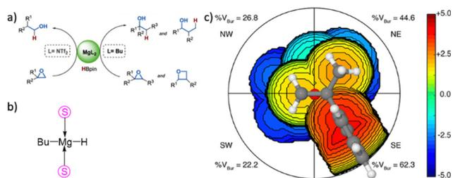
Fig. 7 (a) Regiodivergent ring opening of epoxides. (b) Rate determining intermediate and (c) its steric map including the  $\%V_{\text{Bur}}$  of the quadrants (The origin is set at the midpoint of the C–C bond within the epoxide, and the O atom of the epoxide is positioned along the Z-axis. The scale of the steric contours is included in Å). Adapted with permission.<sup>248</sup> Copyright © 2020, American Chemical Society.
