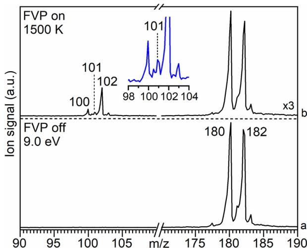
Fig. 2 Molecular beam associated mass spectra of **4** ( $m/z$  180) recorded at a photon energy of 9.0 eV at (a) RT (FVP off) and (b) upon pyrolysis (FVP on) at 1500 K (for details see Fig. S5, ESI<sup>†</sup>). Trace (b) is scaled up by a factor of 3. Inset shows the expansion of the peaks at  $m/z$  100–103.
