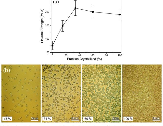
Fig. 5 Effect of crystallization percentage on mechanical properties of a phospho-silicate combeite glass-ceramic. (a) Flexural strength vs. fraction crystallized during a multistage heat treatment schedule. (b) Optical microscope images showing microstructure examples of increasingly crystalized glass-ceramic samples. From ref. 112 with permission from Elsevier, 2001.
