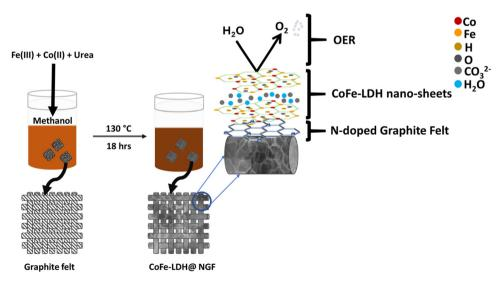
Scheme 1 Schematic illustration for the preparation of the CoFe-LDH@NGF electrode.
