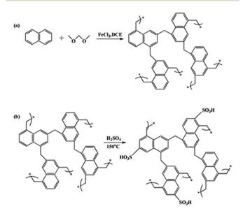
Scheme 1 The structures of the polymer and solid acid. (a) POP-0.01, (b) POP-0.01-SO<sub>3</sub>H-30.
