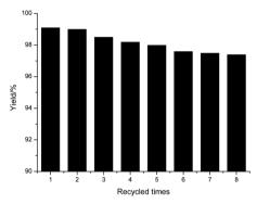
The reuse of POP-0.01-SO<sub>3</sub>H-30 for biodiesel sythesis.
