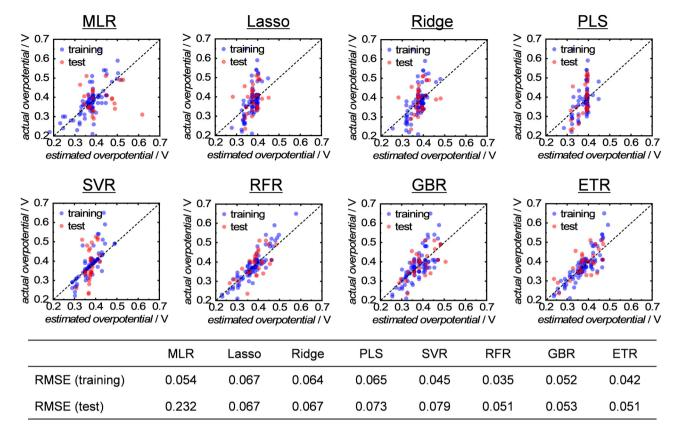
Results of ML analysis with eight types of (non)linear regression models for single-A-site-containing multimetal oxides
