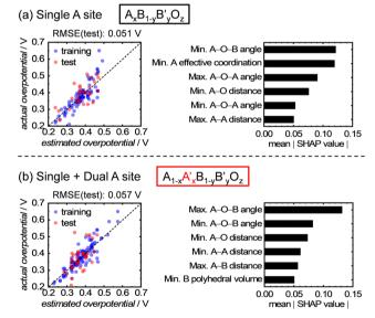
Fig. 5 Comparison of the ML analyses for datasets with (a) only single and (b) single and dual A-site-containing oxides, and the output SHAP values from the ML analysis using the ETR algorithm.
