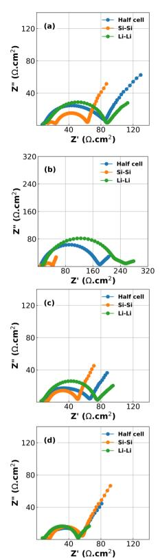
Fig. 1 EIS spectra collected for comparison between half cells and symmetric cells at (a) 0.2 V in the lithiation step; (b) 0.07 V in the lithiation step; (c) 0.3 V in the delithiation step; (d) 0.48 V in the delithiation step.
