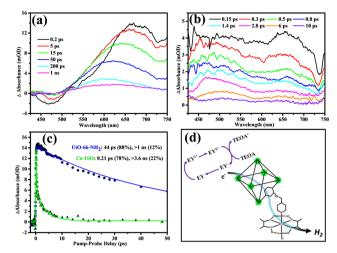
Fig. 4 Ultrafast transient absorption spectral studies of (a) UiO-66-NH<sub>2</sub> and (b) molecular cobaloxime functionalized Co-UiO samples dispersed in the aqueous medium. (c) Comparison of decay kinetics of the two samples at 670 nm. (d) Schematic illustration of the charge transfer path of the Co-UiO catalyst
