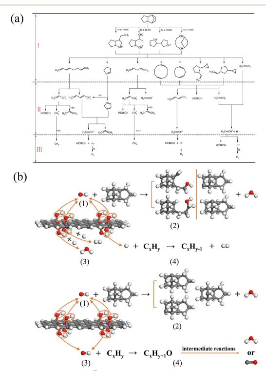
Fig. 4 (a) Three stages of pyrolysis of JP-10 molecules.<sup>19</sup> (b) Pyrolysis and oxidation of JP-10 molecules on functionalized graphene sheets (FGS).<sup>78</sup>
