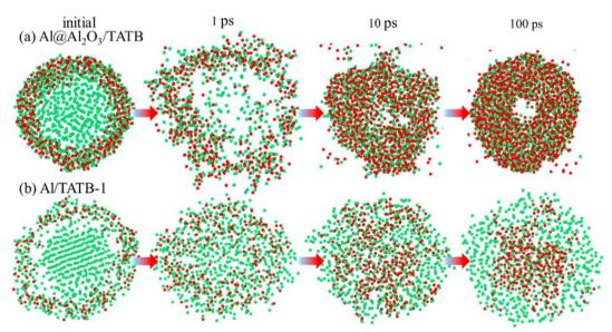
Fig. 10 Morphological evolution of Al atoms in the (a) Al@Al $_2$ O $_3$ /TATB and (b) Al/TATB-1 systems at 3000 K. $^{130}$
