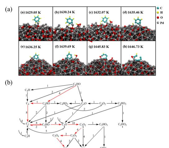
Fig. 3 (a) The oxidation process of C<sub>6</sub>H<sub>6</sub> on Pd nanoparticles and (b) further oxidation of C<sub>6</sub>HO to small molecules.<sup>54</sup>
