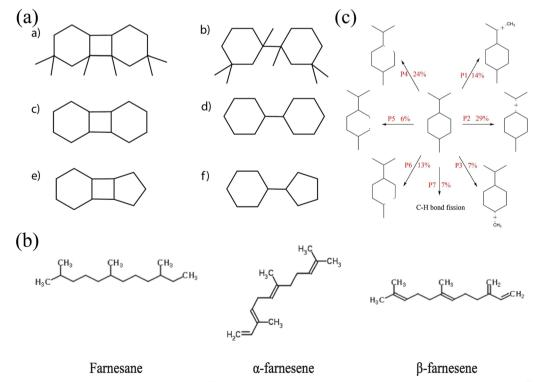
Fig. 5 (a) Molecular structure of six HTH polycyclic alkanes;  $^{80}$  (b) molecular structure of farnesane,  $\alpha$ -farnesane, and  $\beta$ -farnesane,  $^{81}$  and (c) the initial decomposition path and its proportion of PMT molecules.82
