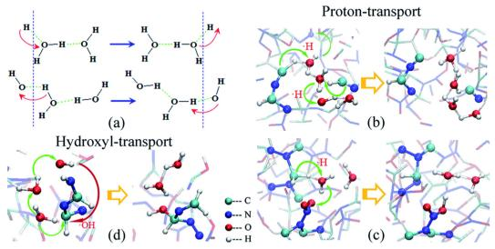
H and OH transport of water in β-HMX: 102 schematic of (a) H and OH transport, (b and c) H transport, and (d) OH transport.
