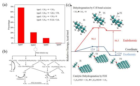
Fig. 2 (a) Four decomposition paths of methylcyclohexane and their proportion;<sup>47</sup> (b) the formation route for the main products of methylcyclohexane;<sup>47</sup> and (c) reaction barriers for the dehydrogenation of MCH with and without added FGS containing an oxygen functional group.<sup>50</sup>
