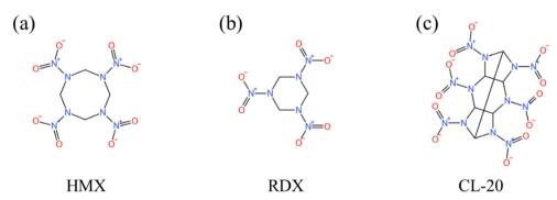
Fig. 7 Molecular structure of (a) HMX, (b) HMX and (c) CL-20.
