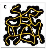
Fig. 8 Schematic diagram showing the effect of filler loading and conductive network formation in carbon black composites, with (a) lower dosage, (b) medium, and (c) optimum loadings of carbon black depicting the percolation thresholds (reproduced with permission from ref. 140 (Copyright 2019, Springer Nature, licensed under a Creative Commons Attribution (CC BY) license)).
