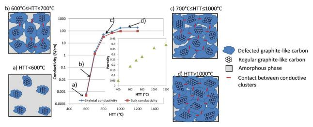
Fig. 7 Scheme describing the conductivity development in biocarbons, reproduced with permission from ref. 138 (Copyright 2018, Elsevier, License number: 5357130750845).
