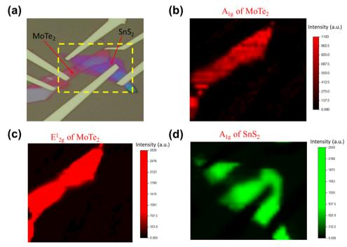
Fig. 2 (a) Optical image of the device that shows the area selected for Raman mapping. (b) Raman intensity maps of  $A_{1g}$  of MoTe<sub>2</sub>. (c) Raman intensity maps of  $E^{1}_{2g}$  of MoTe<sub>2</sub>. (d) Raman intensity maps of  $A_{1g}$  of SnS<sub>2</sub>. Graphical representation of Raman intensity mapping at 172.43 and 232.93 cm<sup>-1</sup> for MoTe<sub>2</sub>, and 315.78 cm<sup>-1</sup> for SnS<sub>2</sub>.
