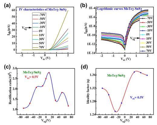
Fig. 4 (a)  $I_{ds}$  –  $V_{ds}$  characteristic curves of the MoTe<sub>2</sub>–SnS<sub>2</sub> heterostructure at various back gate voltages ( $V_{bq}$ ); the linear scale. (b) Logarithmic scale. The maximum rectification ratio is  $2.79 \times 10^5$  mA W<sup>-1</sup>. (c) The change in the rectification ratio of the device at various back gate voltages. (d) The variation in the ideality factor at different gate voltages.
