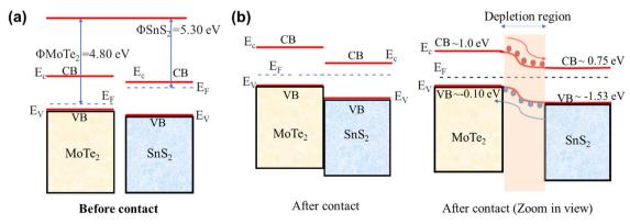
Fig. 5 Schematic illustration of the band diagram for the p-MoTe<sub>2</sub>/n-SnS<sub>2</sub> structure-based diode at  $V_{bq} = 0 \text{ V}$ . (a) Schematic signifies the band diagram of a p-MoTe<sub>2</sub>/n-SnS<sub>2</sub> diode before connection, and (b) symbolizes the diode after connection.
