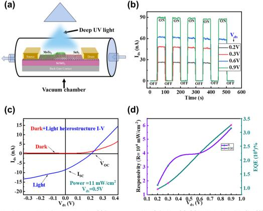
Fig. 6 (a) Schematic of the p-n device for photodetection. (b) Photocurrent at  $V_q = 0$ , for  $V_{ds} = 0.2 - 0.9$  V with incident light ( $\lambda = 220$  nm) and power intensity 11 mA cm<sup>-2</sup>. (c) I-V curves in the dark and under light, representing  $I_{SC} = -8.5$  nA and  $V_{OC} = 0.20$  V at  $V_{q} = 0$ . (d) The change in responsivity at different values of  $V_{\rm ds}$ . (e) The enhancement in the EQE at different values of  $V_{\rm ds}$ .
