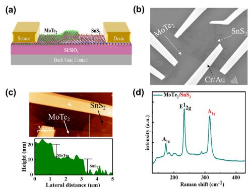
Fig. 1 (a) Schematic illustration of the p-n device. (b) SEM image of the p-n heterostructure  $MoTe_2-SnS_2$ -based device; the scale bar is 5  $\mu$ m. (c) AFM profile of the heterostructure. (d) Raman spectra of the  $MoTe_2-SnS_2$  heterostructure.
