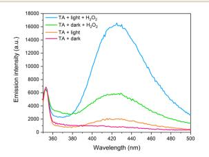
Fig. 10 Photoluminescence emission spectra of hydroxyterephthalic acid generated using LDH/BNOx catalyst.
