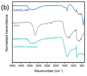
Fig. 1 (a) pXRD patterns and (b) FT-IR spectra of CuAl-CO<sub>3</sub> LDHs (blue), BNOx (grey) and LDH/BNOx nanocomposite (turquoise). pXRD reference patterns are provided for CuAl hydrotalcite, boron nitride and boric acid.
