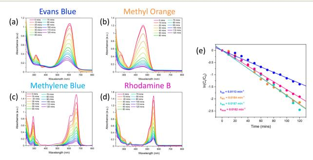
Fig. 7 Reduction in UV-vis absorbance of (a) Evans blue, (b) methyl orange, (c) methylene blue and (d) rhodamine B by visible-light photo-degradation in the presence of LDH/BNOx membrane catalysts and 10  $\mu$ L of H<sub>2</sub>O<sub>2</sub> (30% w/w). (e) PFO models for degradation of Evans blue, methyl orange, methylene blue and rhodamine B.
