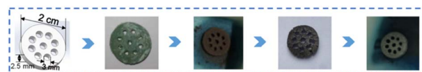
Fig. 4 Printed ceramic electrode Ti-Ni NS obtained by digital light printing technology after degreasing, sintering, and reduction, respectively [reproduced from ref. 26, with kind permission].
