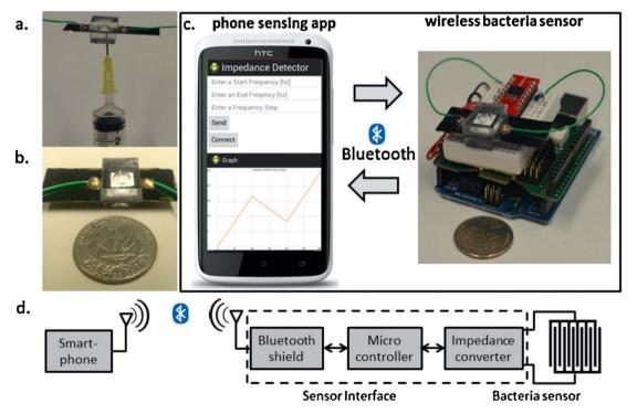
Fig. 3 Smartphone based wireless bacteria sensing device (a) syringe to inject testing sample in the senor, (b) EIS based bacteria sensing (c) communication between smartphone and sensor device for bacteria sensing, (d) wireless circuit system.<sup>76</sup>
