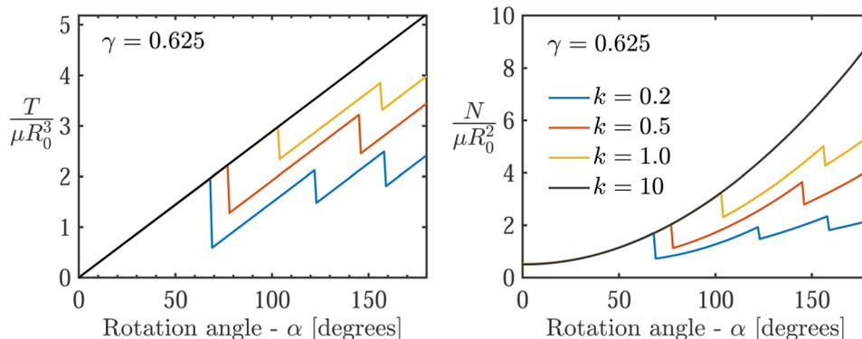
Fig. 6 The evolution of dimensionless torque (left) and corresponding normal force (right) with respect to rotation angle, for various values of  $k$ . Here we use  $\gamma = 0.625$ ,  $R_0/H = 1$ , and the initially applied dimensionless normal force is set to 0.5.
