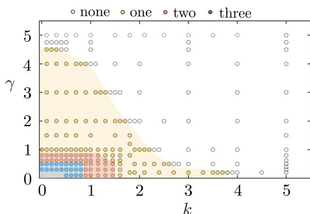
Fig. 7 Phase portrait showing the number of stick-slip events that occur for rotation of  $\alpha = 180$  degrees, as a function of the dimensionless material properties ( $k, \gamma$ ). Different shaded regions correspond to different numbers of delamination events, as identified from theoretical predictions, indicated via circular markers. The gray region corresponds to situations in which the number of snap-through events is greater than 4.
