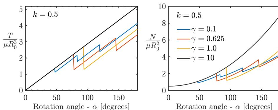
Fig. 5 The evolution of dimensionless torque (left) and corresponding normal force (right) with respect to rotation angle, for various values of  $\gamma$ . Here we use  $k = 0.5$ ,  $R_0/H = 1$ , and the initially applied dimensionless normal force is set to 0.5.
