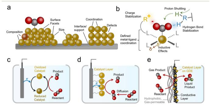
Fig. 2 The diversity of active sites within heterogeneous electrocatalysts (a) contrasts with the well-defined catalytic sites and functional environments of molecular systems (b). Molecular catalysts can function as solubilized species (c) or heterogenized on electrode surfaces (d) or within gas-diffusion electrodes (e).
