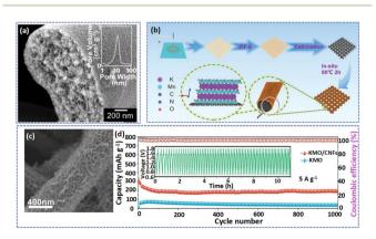
Fig. 4 (a) Cross-sectional SEM image of a porous carbon fiber. Adapted from ref. 68, copyright 2022, Wiley-VCH. (b) The fabrication of KMO/CNFs is illustrated schematically. (c) SEM image of KMO/CNFs. (d) Long-term cycling performance of KMO/CNFs at 3.0 A  $\rm g^{-1}$ . Adapted from ref. 106, copyright 2022, Wiley-VCH.
