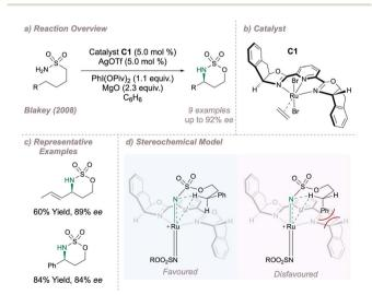
Fig. 10 Application of a Ru-(PyBOX) complex for asymmetric intramolecular  $C(sp^3)$ -H amination.
