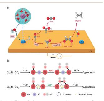
Fig. 5 (a) Schematic illustration of the possible reaction mechanism for  $C_2H_4$  generation over F–Cu catalysts. The purple, blue, red, gray, and white spheres represent K, F, O, C, and H atoms, respectively. Reproduced from ref. 93. Copyright 2020 Nature. (b) Schematic illustration of the simplified ECR mechanism towards  $C_2$  products demonstrated by the  $Cu_3N_x$  model with nitrogen vacancies. Reproduced from ref. 122. Copyright 2021 Wiley-VCH.
