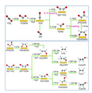
Fig. 3 Possible C–C coupling mechanisms in the electrocatalytic  $CO_2$  reduction (above). Mechanisms of forming  $C_2H_4$  and  $C_2H_5OH$  after C–C coupling (below). Reproduced from ref. 92. Copyright 2021 Royal Society of Chemistry.
