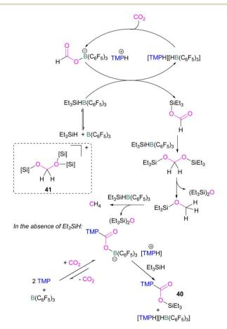
Scheme 27 Converting stoichiometric  $CO_2$  reduction into a catalytic process by adding excess  $B(C_6F_5)_3$  and  $Et_3SiH$  to the TMP/ $B(C_6F_5)_3$  FLP system.
