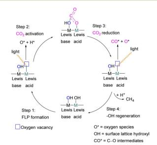
Scheme 67 Heterogenous Ge FLP in the reduction of  $CO_2$  to  $CH_4$ . M = Metallic element.
