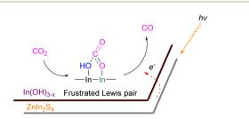
Fig. 11 An FLP  $Znln_2S_4/ln(OH)_3 = x$  (ZIOS) heterojunction system for the reduction of CO2 to CO.
