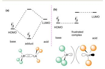
Fig. 3 Frontier molecular orbital presentation of (a) a classic Lewis acid-base adduct and (b) a frustrated Lewis pair. LA = Lewis acid; LB = Lewis base.
