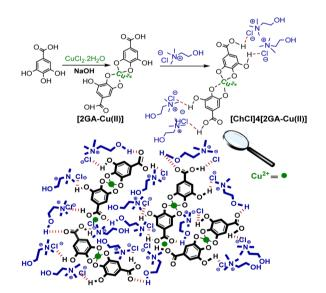
Scheme 2 The suggested illustration of molecular structure of [2GA-Cu( $\shortparallel$ )] complex and also possible interactions between [2GA-Cu( $\shortparallel$ )] complex and choline chloride (ChCl).
