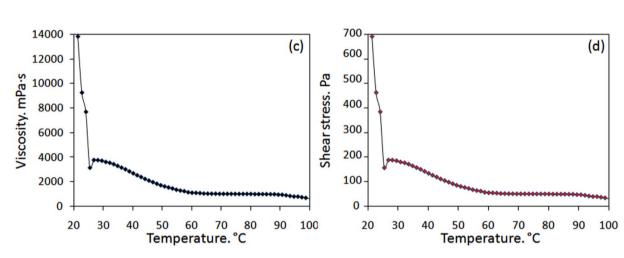
Fig. 5 (a) Viscosity *versus* shear rate at 50 °C and (b) shear stress *versus* shear rate at 50 °C of [ChCl]<sub>4</sub>[2GA-Cu( $\parallel$ )]; (c) dependence viscosity *versus* temperature, and (d) dependence shear stress *versus* temperature at shear rate 50 s<sup>-1</sup> of [ChCl]<sub>4</sub>[2GA-Cu( $\parallel$ )].
