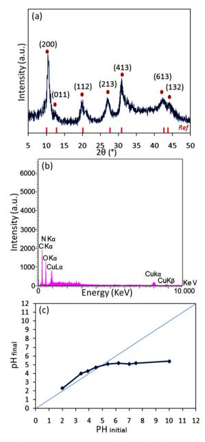
Fig. 2 (a) Powder X-ray diffraction of [2GA-Cu( $\parallel$ )]; (b) EDX analysis of [2GA-Cu( $\parallel$ )]; (c) pH<sub>pzc</sub> determination graph of [2GA-Cu( $\parallel$ )].
