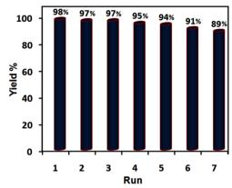
Fig. 9 Evaluating recyclability and reusability of [ChCl] $_4$ [2GA-Cu( $_1$ )] in the synthesis of 1-benzyl-4-phenyl-1H-triazole under the optimized conditions.
