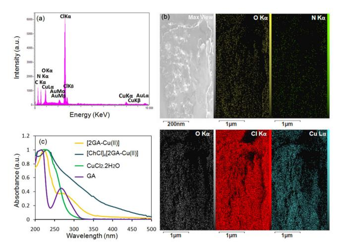
Fig. 4 (a) EDX analysis; (b) mapping images of the constructing elements of [ChCl]<sub>4</sub>[2GA-Cu( $\shortparallel$ )]; (c) UV-Vis normalized spectra of CuCl<sub>2</sub>·2H<sub>2</sub>O, GA, [2GA-Cu( $\shortparallel$ )], and [ChCl]<sub>4</sub>[2GA-Cu( $\shortparallel$ )] in deionized water (0.0005 M).
