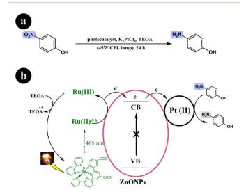
Scheme 16 Reaction conditions and (b) diagrammatic representation that elucidates the potential mechanism underlying the photoreduction process of *p*-nitrophenol into *p*-aminophenol. Reproduced from ref. 52, with permission, copyright 2015, Royal Society of Chemistry.
