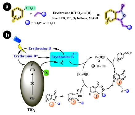
Scheme 25 (a) Reaction conditions and (b) catalytic activation of C-H bonds facilitated by Ru(II) and photoredox using  $O_2$  as an oxidant under blue LED irradiation. Reproduced with permission from ref. 75. Copyright 2020, John Wiley and Sons.
