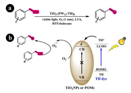
Scheme 21 (a) Reaction conditions for the aerobic oxidation of aryl alcohols to aldehydes by  $TiO_2$ -(PW<sub>12</sub>-TH)<sub>8</sub> under Blue light irradiation; (b) mechanistic pathway. Reproduced with permission from ref. 64, copyright 2017, Elsevier.
