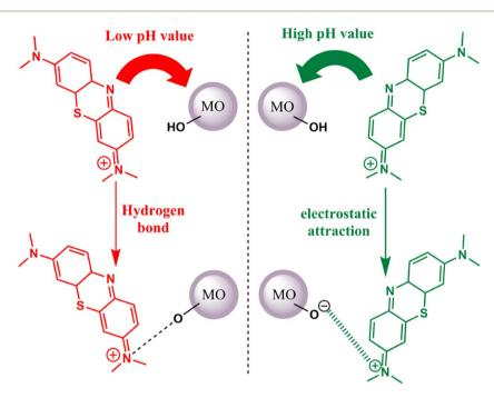
Fig. 4 Possible interactions between the TH dye and metal oxides at low pH (hydrogen bonding) and high pH (electrostatic attraction). Adapted with permission from ref. 63, copyright 2018, Elsevier.
