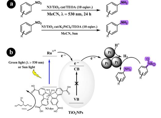
Scheme 14 (a) Reaction condition for the conversion of nitroarenes to anilines and (b) the proposed mechanism involving the reduction of nitroarenes using a green-light/sun light mediated process facilitated by dye-sensitized TiO2 and transition metal clusters. TEOA (triethanolamine) is also involved in the reaction. Reproduced from ref. 55 with permission, copyright 2010, Royal Society of Chemistry.
