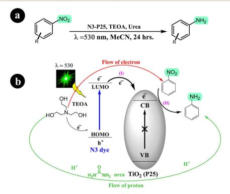
Scheme 15 (a) The conversion reaction and the conditions for the catalysis system; (b) the reduction of nitrobenzene through photocatalysis using dye-sensitized  $TiO_2$  is achieved in the presence of urea, which acts as a mediator for proton transfer. Reproduced from ref. 56 with permission, copyright 2011, Royal Society of Chemistry.
