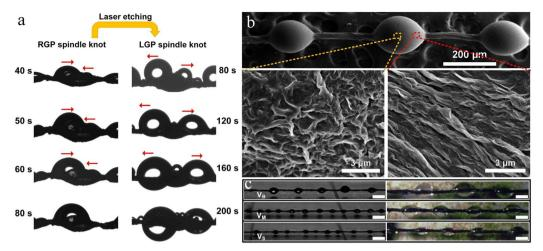
Fig. 9 (a) Through changing the surface wettability of the spindle knot, the movement direction of water droplets could be controlled; (b) SEM images of individual spindle knots; (c) optical and stereomicroscope images of spindle knots of different sizes.  $^{36}$  Scale: (c) 200  $\mu$ m. This figure has been adapted from ref. 36 with permission from Nature Portfolio, 2017.
