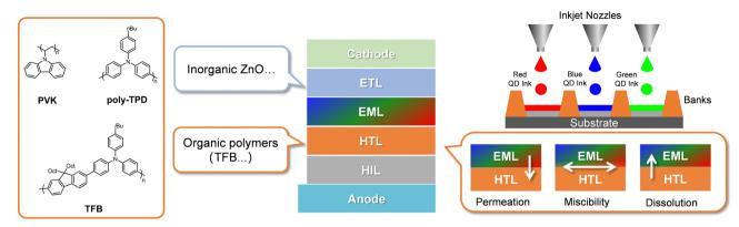
Fig. 2 Challenges in solution-processable HTM-based IJP QD-LEDs.
