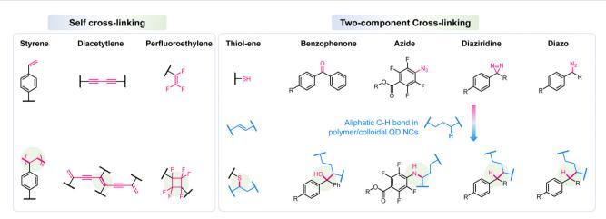
Fig. 1 The fundamental chemistries of the current cross-linking strategies used in QD-LEDs.
