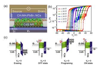
Fig. 13 (a) Schematic device structure of MAPbBr<sub>3</sub> NCs/CdS NR memory transistor. (b) Electrical transfer characteristics at  $V_{\rm DS}$  = 1 V of the device recorded after every sweeping cycle. (c) Energy band diagrams of the device during the charge storage process. Reproduced with permission.<sup>207</sup> Copyright © 2019, American Chemical Society
