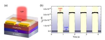
Fig. 12 (a) Schematic structure illustration of the phototransistor with an MAPbl<sub>3</sub> channel. (b) Photocurrent responses of the phototransistors on light illumination, showing time-dependent photosensitivity with a time interval of 0.5 s at  $V_{\rm GS}$  = -30 V and  $V_{\rm DS}$  = -30 V. Reproduced with permission.<sup>172</sup> Copyright © 2015, Feng Li et al.
