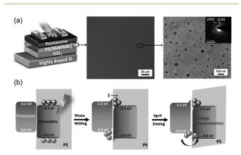
Fig. 14 (a) Schematic device configuration of the PS with dispersed MAPbBr3 NCs photomemory with the SEM and TEM images of the MAPbBr<sub>3</sub>/PS composite film. (b) The operating mechanism of the nonvolatile perovskite-based photomemory. Reproduced with permission.<sup>210</sup> Copyright © 2017, John Wiley & Sons.
