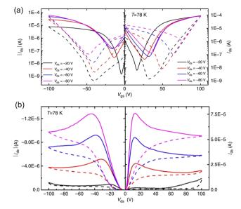
Fig. 6 Ambipolar transport characteristic of the perovskite FET at low temperature. Transfer (a) and output (b) characteristics were tested at 78 K. Solid and dashed curves are measured with forward and backward sweeping, respectively. Reproduced with permission. 108 Copyright © 2015. Xin Yu Chin et al.
