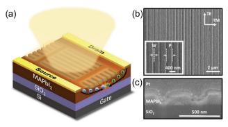
Fig. 17 (a) Schematic illustration of a perovskite LET with a metasurface. (b) Top-view and (c) cross-sectional SEM images of a MAPbI<sub>3</sub> perovskite metasurface film. The inset picture in (b) shows the geometrical parameters of the metasurface structure, including the groove width (W) and nanograting period (P). Reproduced with permission. <sup>233</sup> Copyright © 2022 John Wiley & Sons.
