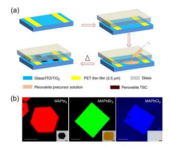
Fig. 7 (a) Schematic illustration of spatially confined inverse temperature crystallization method for producing thin single crystals (TSCs). (b) Fluorescence microscopy images of MAPbI<sub>3</sub>, MAPbBr<sub>3</sub>, and MAPbCl<sub>3</sub> TSCs, respectively. Reproduced with permission. 23 Copyright © 2018, Weili Yu et al.
