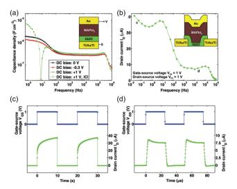
Fig. 18 (a) Capacitance densities at different DC operating conditions. (b)  $I_{\rm D}$  as a function of the  $V_{\rm GS}$  frequency. (c) and (d)  $I_{\rm D}$  response at  $V_{\rm GS}$  frequency of (c) 0.05 Hz and (d) 20 kHz. Reproduced with permission.<sup>241</sup> Copyright © 2018, John Wiley & Sons.
