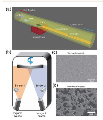
Fig. 4 (a) Synthesis of MAPbCl<sub>3</sub> by the CVD method. MACl and PbCl<sub>2</sub> sources were placed in different places in a single CVD tube. Reproduced with permission.84 Copyright © 2015, American Chemical Society. (b) Schematic illustration of the dual-source thermal evaporation system. (c) and (d) SEM top views of a vapor-deposited perovskite film (c) and a solution-processed perovskite film (d). Reproduced with permission.<sup>85</sup> Copyright © 2013, Springer Nature.
