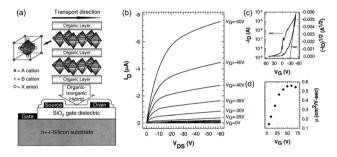
Fig. 8 Structure and properties of the first perovskite-based FET. (a) Schematic illustration of the (PEA)<sub>2</sub>SnI<sub>4</sub> FET. (b) and (c) Output (b) and transfer (c) curves of the transistor. (d) The variation of mobility versus gate voltage. Reproduced with permission. 18 Copyright © 1999, AAAS.
