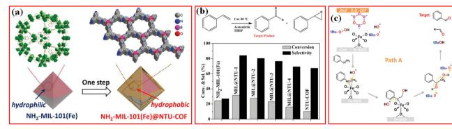
Fig. 12 (a) Fabrication of NH<sub>2</sub>-MIL-101(Fe)@NTU-COF; (b) Styrene oxidation reaction catalyzed by different catalysts using TBHP as the oxidant; (c) proposed mechanism path A for styrene transformed to benzaldehyde. Reproduced with permission.<sup>21</sup> Copyright 2019, Wiley-VCH.
