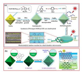
Fig. 9 (a) Schematic scope of the preparation of Pd-doped TiATA@LZU1 core-shell and their photocatalytic applications in batch and dualchamber microreactor. Reproduced with permission.<sup>69</sup> Copyright 2018, Wiley-VCH. (b) Illustration of the preparation of Ti-MOF@Pt@DM-LZU1 and photocatalytic mechanism. Reproduced with permission. <sup>66</sup> Copyright 2020, ACS Publishing Group.
