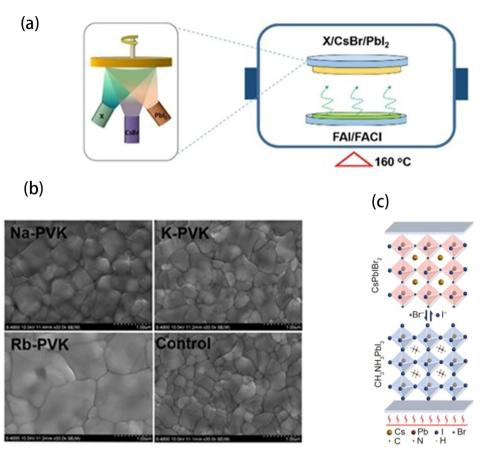
Fig. 10 (a) Schematic illustration of the vapor-solid reaction process. (b) SEM images of the control, Na-PVK, K-PVK, and Rb-PVK films. Reproduced from ref. 113 with permission from Wiley-VCH, copyright 2021. (c) Schematic illustration of the halide exchange strategy with a slow reaction rate. Reproduced from ref. 115 with permission from Springer Nature, copyright 2021.
