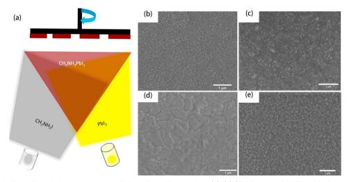
Fig. 11 (a) Schematic illustration of the pressure-controlled co-deposition method. (b)-(e) SEM images of MAPbl<sub>3</sub> thin films prepared at different pressures. (b)  $7.5 \pm 0.3 \times 10^{-4}$  Pa (125 °C), (c)  $1.5 \pm 0.3 \times 10^{-3}$  Pa (150 °C), (d)  $4.5 \pm 0.3 \times 10^{-3}$  Pa (175 °C), and (e)  $7.5 \pm 0.3 \times 10^{-3}$  Pa (175 °C). The scale bar is  $1 \mu m$ . Reproduced from ref. 120 with permission from Elsevier, copyright 2019.
