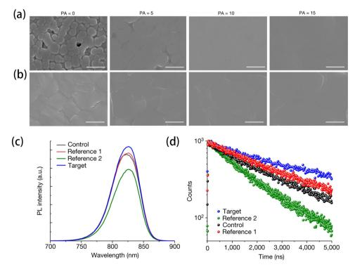
Fig. 7 SEM images of the surface morphologies of the perovskite thin films spin-coated with 0-15 mol% PACl added to the FAPbl<sub>3</sub> precursor containing 35 mol% MACI (a) without annealing and (b) with annealing. The scale bar is 1.0 µm. (c) Photoluminescence (PL) and (d) time-resolved photoluminescence (TRPL) spectra of the perovskite films deposited on a glass substrate. Reproduced from ref. 32 with permission from Springer Nature, copyright 2023.
