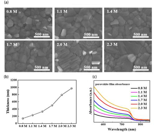
Fig. 4 (a) SEM images of the perovskite films with various precursor concentrations. The scale bar is 500 nm. (b) Thickness of perovskite films and (c) absorption spectra of perovskite films with various precursor concentrations. Reproduced from ref. 72 with permission from Multidisciplinary Digital Publishing Institute, copyright 2022.
