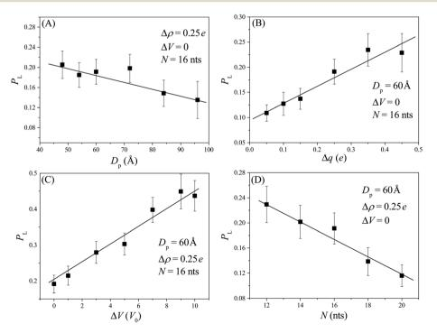
Fig. 2 The successful landing probability  $P_L$  of the nanorobot as a function of pore-pore distance  $D_P$  (A), pore charge gradient  $\Delta q$  (B), external voltage  $\Delta V$  (C), and the leg length N (D). The lines serve as a visual guide. It should be noted that the data point at  $D_p$  = 96 Å presented in panel (A) is an average of 40 samples due to the long computational time required.
