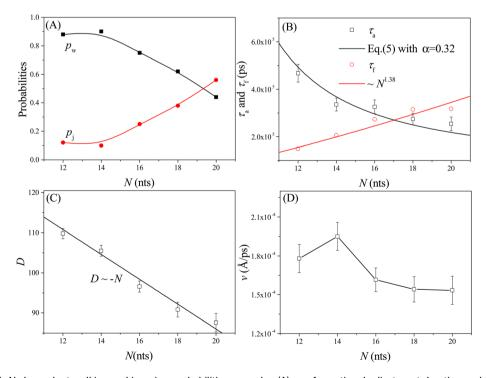
Fig. 8 The leg length N-dependent walking and jumping probabilities  $p_w$  and  $p_j$  (A), conformational adjustment duration and forward-moving duration  $\tau_a$  and  $\tau_f$  (B), moving distance D of the nanorobot from the state F2 to the state F4 (C), and moving velocity v from all simulation samples (D). Here  $D_p = 60$  Å,  $\Delta q = 0.25e$ , and  $\Delta V = 0$ .
