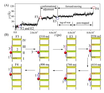
Fig. 7 (A) The time-evolutional trace of the nanoparticle along y-direction at  $D_p = 60$  Å,  $\Delta q = 0.25e$ , and  $\Delta V = 10V_0$ . (B) The snapshots of the nanorobot in the step III-IV (from the state F3 to state F4). In order to clearly discriminate the three legs of the nanorobot in different states, leg1, leg2, and leg3 are highlighted by blue, green, and magenta, respectively.
