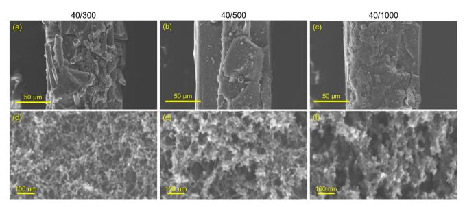
Fig. 1 Scanning electron micrographs of 1-ply CNFP cross-sections for CNFP-40/300 (a), CNFP-40/500 (b), and CNFP-40/1000 (c), and their respective magnified images (d-f). In (a-c), the carbon nanofoam appears as a solid filling the gaps in the carbon fiber paper, and the pores are only visible at much higher magnifications (d-f).
