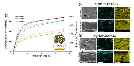
Fig. 3 (a) Mass uptake by CNFPs upon vapor infiltration of  $S_8$  as a function of time: solid line represents the measured mass uptake in the CNFP, and the dotted line shows the mass of S<sub>8</sub> uptake relative to the carbon nanofoam component of the CNFP. Scanning electron microscopy and cross-sectional EDS analysis of C and S for (b) 2 h and (c) 6 h infiltrations.
