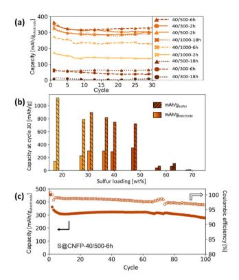
Fig. 5 (a) Summary of Li-S cycling capacities at 0.1C for CNFPs using different sulfur infiltration durations and (b) their corresponding gravimetric capacities per weight sulfur and per total electrode weight after cycle 30 versus their sulfur weight loadings. (c) Long-term cycling of the S@CNFP-40/500-6 h sample to 100 cycles. Results are summarized in Table S4,† and cycling capacity normalized to sulfur mass is shown in Fia. S5.†
