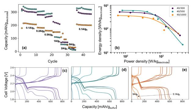
Fig. 6 (a) Rate study of Li–S coin cells from 0.1 A  $g_{sulfur}^{-1}$  to 5 A  $g_{sulfur}^{-1}$ , (b) the Ragone plot produced from the third cycle of each rate, and (c–e) their corresponding charge–discharge curves.
