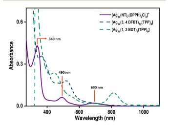
Fig. 2 The UV-vis spectra of  $[Ag_{14}(NT)_7(DPPH)_2Cl_2]^+$  (violet trace),  $Ag_{14}(3,4$  DFBT) $_{12}TPP_8$  (dark blue trace), and  $Ag_{14}(1,2$  BDT) $_6TPP_8$  (sea green trace).
