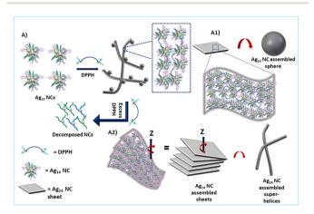
Scheme 1 Schematic illustration showing the mechanism of DPPHinduced orthogonal self-assembly of Aq14 NCs into superhelices and spheres.
