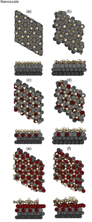
Fig. 5 Top and side views of model structures for the most stable phases: (a) 4  $\times$  4 and (b)  $\sqrt{13}\times\sqrt{13}$  on Ag(111); (c and d) the same on Ag<sub>2</sub>Sn–Ag(111); (e) TDS and (f) HDS  $\sqrt{3}\times\sqrt{3}$  on Sn–Ag(111). Si atoms are represented as yellow spheres, Sn as red and Ag as gray ones; darker colors are used for deeper atoms.
