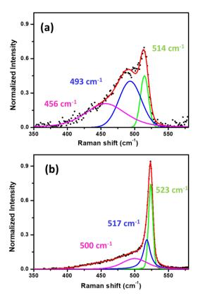
Fig. 3 Raman spectra obtained from: (a) 1 ML and (b) 6 ML deposited on Ag<sub>2</sub>Sn-Ag(111) template. The black-dotted curves are the as acquired raw spectra, red curves are the fitted spectra where the green, blue and purple are three fitted Lorentzian-Gaussian components following the background subtraction.
