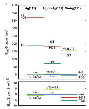
Fig. 4 (a) Adsorption energy per Si atom of different silicene reconstructions on the Ag(111), Ag<sub>2</sub>Sn-Ag(111) and Sn-Ag(111) substrates. Values are referred to the  $4 \times 4$  case. (b) Enlargement of the most stable
