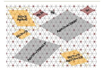
Fig. 2 Ag(111) surface lattice (gray lines) showing tin atoms of Ag<sub>2</sub>Sn (brown circles), unit cells of Ag(111) (small gray area), Ag<sub>2</sub>Sn-Ag(111) and Sn-Ag(111) (brown areas), silicon structures (yellow areas), and Ag supercells used in the calculations (large gray areas).
