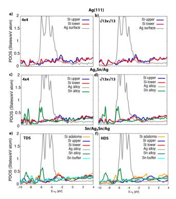
**Fig. 6** Density of states, resolved for chemical species, of the most stable phases on different substrates: (a)  $4\times4$  and (b)  $\sqrt{13}\times\sqrt{13}$  on Ag(111); (c and d) the same on Ag<sub>2</sub>Sn-Ag(111); (e) TDS and (f) HDS on Sn-Ag(111).
